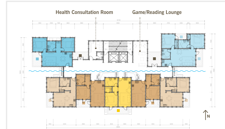
Upper Floor (typical) Majority of units on each floor retain solar heat gain from the south-facing orientation, with the largest units positioned independently on the corners.
