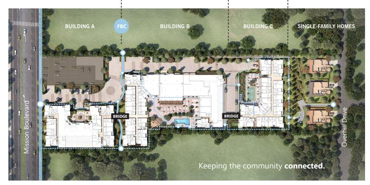
Site Plan: Physical site constraints and Form-based Code requirements dictate the organization of development into three building blocks with pathways that traverse, cross and loop throughout the community. Building-to-building bridges offer elevated connections directly from the upper floors.
